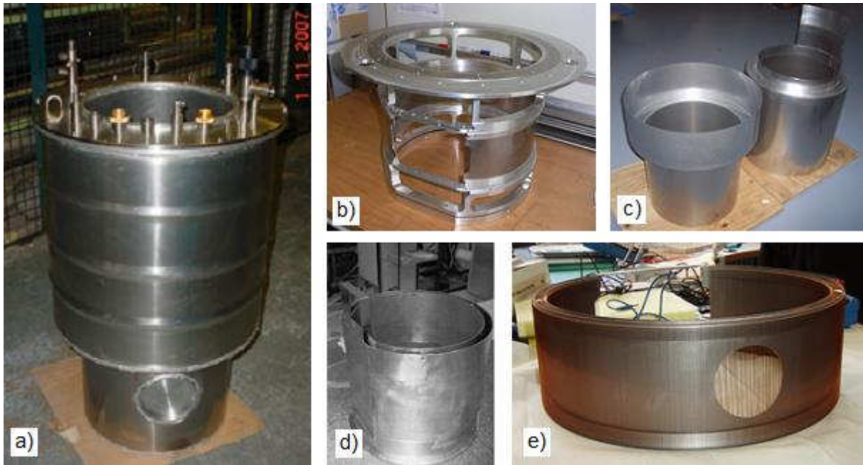
FIG. 1. Main components of the new Cryopad produced by different companies; a) cryostat made by AS Scientific, Oxfordshire, UK, b) precession coils frame made at IFF workshop FZ Jülich, Germany c) \mu -metal shields made by Magnetic Shields Ltd, Kent, UK, d) Nb Meissner screens produced by SDMS, Saint-Romans, France, e) outgoing superconducting precession coil wound at ILL, France.
